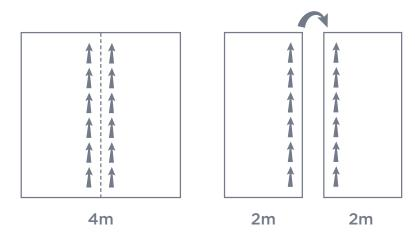
If more than one roll of the same colour is required, all the rolls must be from the same batch and installed in the same order as they are numbered. Beauflor cannot guarantee a colour match between different batches.
