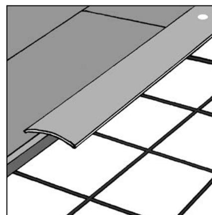
Figure 23 Threshold strip
