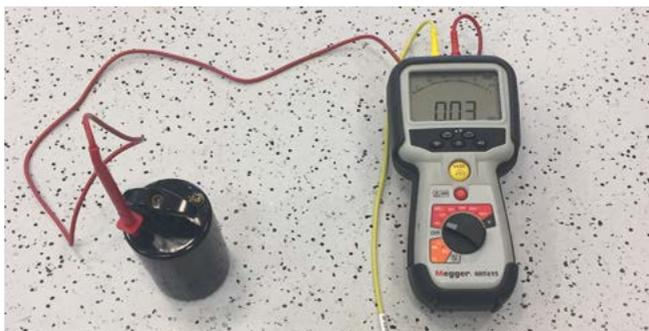
Figure 3 Test electrode with an insulation tester
